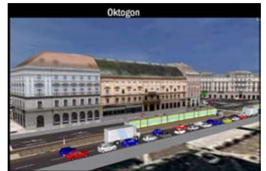
Computerized (Vissim) traffic model of one of the partial networks of Budapest
