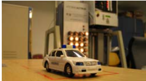
Public road traffic control equipment with "miniloop" vehicle loop detector
