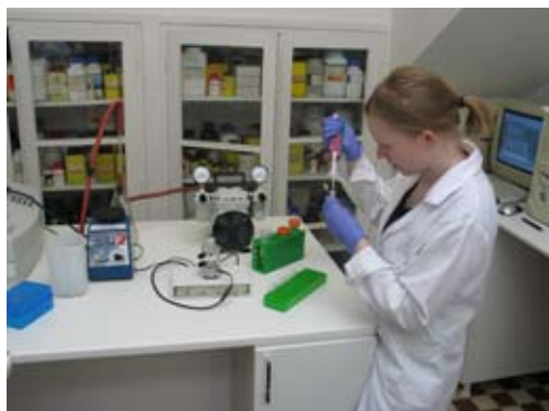
Respiration analysis with a Clark electrode
