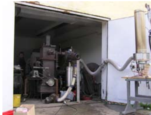
On-site analytical measurement of biomass gasification
